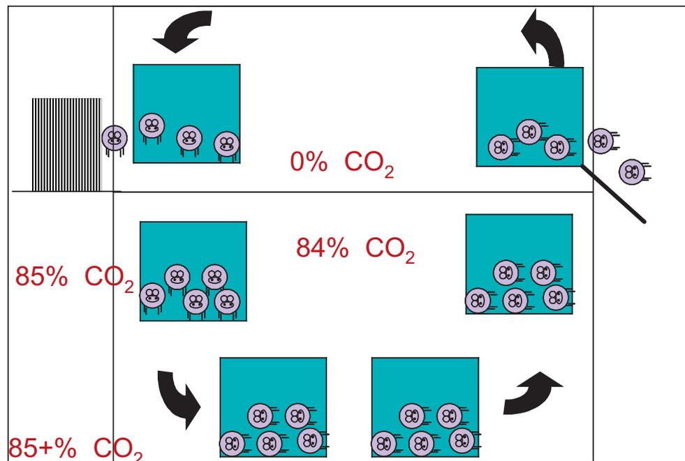
**Figure 1 - Example of side-entry carbon dioxide stunning machine**
