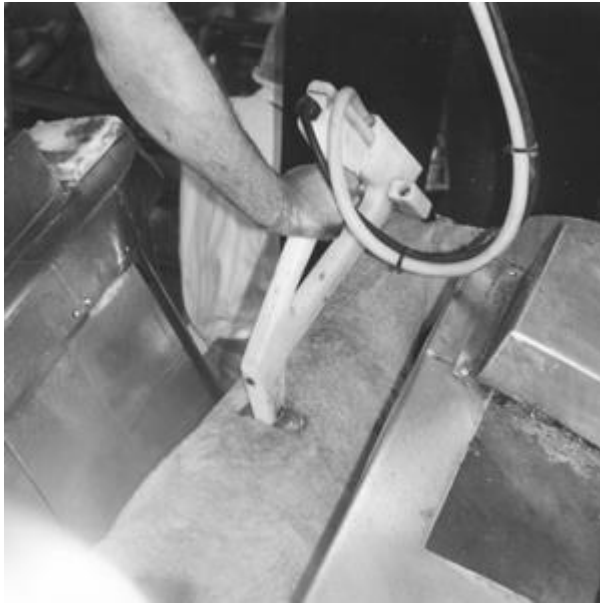
Figure 14 Correct back electrode positioning
