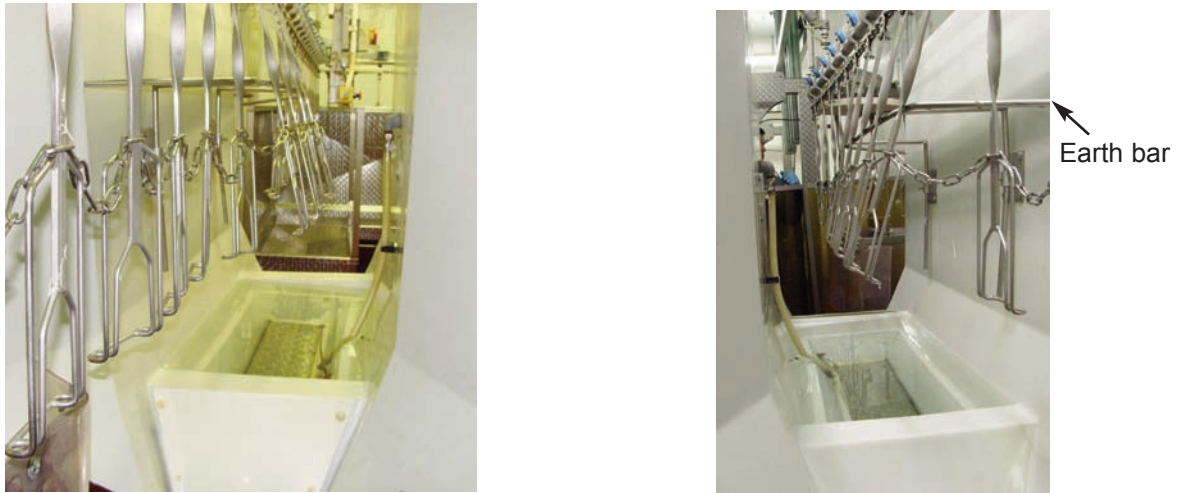
Figure 21. The entrance (left) and exit (right) of a waterbath stunner. The shackles are pushed out by the earthed rubbing bar, to enable continuous electrical contact.
