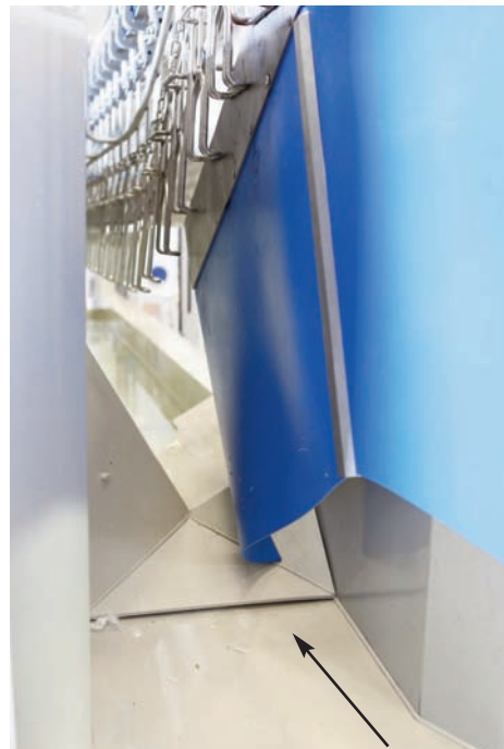
Figure 7b. An alternative design of entry ramp, where the edge has a section cut-away which causes a bird's head to drop through the opening, into the water, before the body and wings. Such ramps may need to be made-to-measure, to cater for the bird type being processed. The arrows indicate the direction of bird conveyance. Image on left: HSA (2006). Image on right: Marel Stork Poultry Processing.
