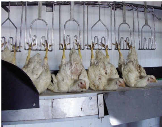
Figure 4. Broiler chickens and turkeys atop a breast support conveyor. The conveyor advances at the same speed as the shackle line. Once each bird is shackled and sitting appropriately upon the conveyor, the shackler should fold the birds' wings into the natural closed position, to reduce the risk of pre-stun shocks.
