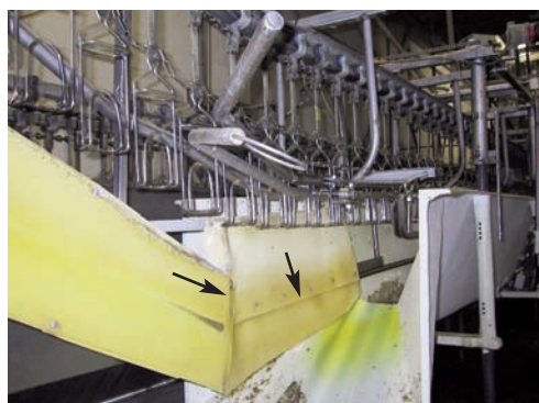
Figure 3b. Breast contact strips should extend up to the waterbath entrance, as shown in this image. Contact strips should be made of one piece of material and should not have joints that may disturb birds as they move over it. This image shows two joints (indicated by arrows) which are not smooth and should be replaced with a single piece of material.
