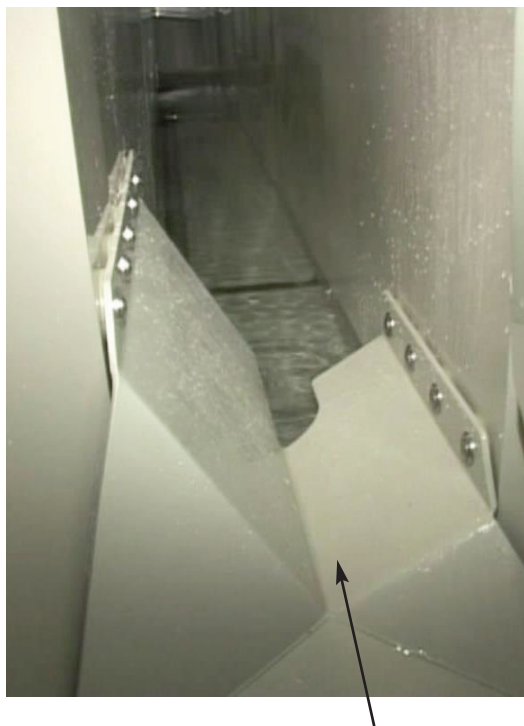
Figure 7b. An alternative design of entry ramp, where the edge has a section cut-away which causes a bird's head to drop through the opening, into the water, before the body and wings. Such ramps may need to be made-to-measure, to cater for the bird type being processed. The arrows indicate the direction of bird conveyance. Image on left: HSA (2006). Image on right: Marel Stork Poultry Processing.
