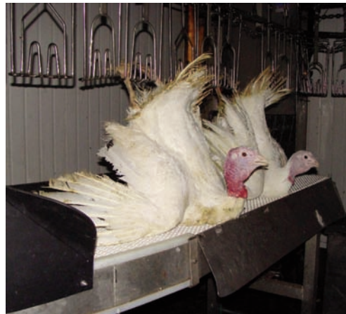
Figure 4. Broiler chickens and turkeys atop a breast support conveyor. The conveyor advances at the same speed as the shackle line. Once each bird is shackled and sitting appropriately upon the conveyor, the shackler should fold the birds' wings into the natural closed position, to reduce the risk of pre-stun shocks.
